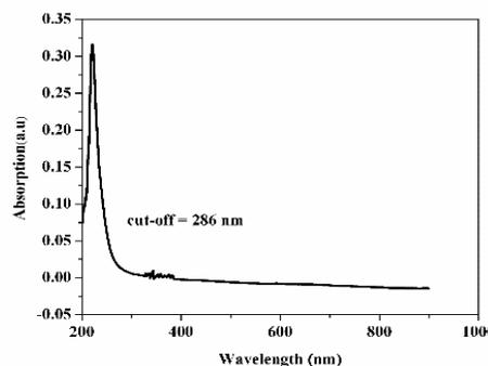
Fig. 6. UV- vis absorption spectra of GSQ crystal
