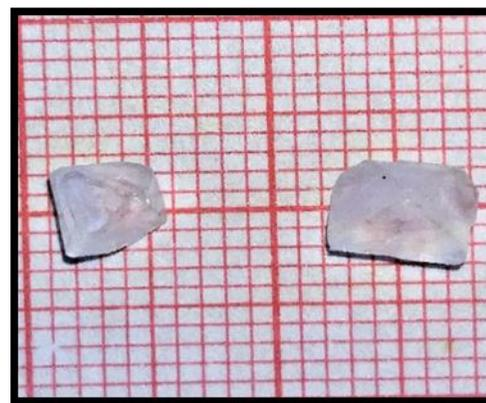
**Fig. 1.** Photograph of as grown GSQ single crystal.
