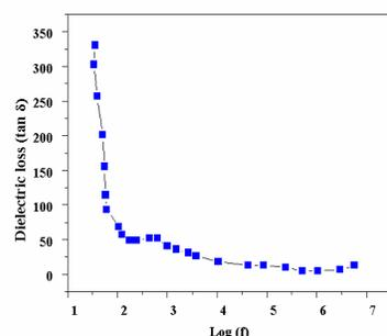
**Fig. 10.** Variation of dielectric constant with frequency of GSQ crystal
