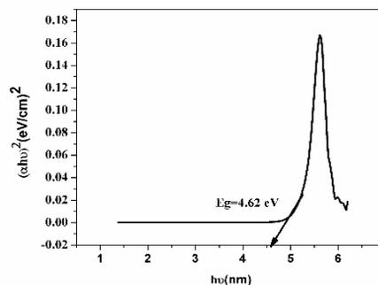
Fig. 7. UV- vis bandgap of GSQ crystal
