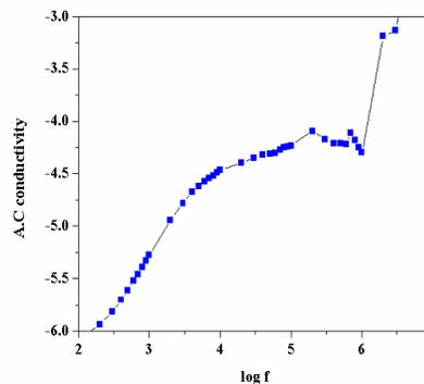
**Fig. 11.** Variation of A.C. conductivity with frequency of GSQ crystal
