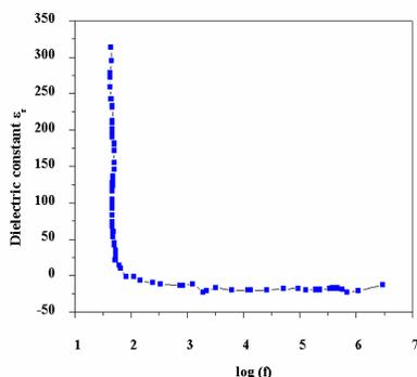
**Fig. 9.** Variation of dielectric constant with frequency of GSQ crystal
