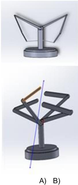
**Fig 3** Cartesian space trajectory: a) robot run into itself in Cartesian space, b) change in joint angles [20].
