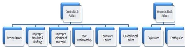
Fig. 1 Controllable & Uncontrollable Failure.
