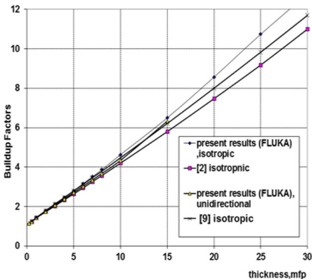
Fig. 6. Comparison of Exposure Buildup Factors of photon in Concrete for a point isotropic photon source (FLUKA) with an energy of 10 MeV obtained in different literatures
