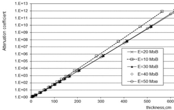
**Fig. 5.** Dependence of the attenuation coefficient of the absorbed dose in Concrete on the shielding thickness for point isotropic photon sources with different initial energy
