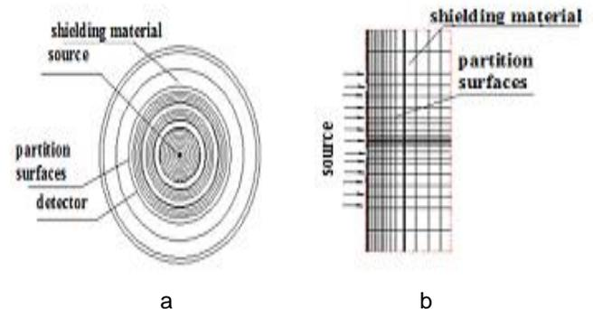
**Fig. 1.** Geometries of the considered compositions: a) – point source, b) – unidirectional source)
