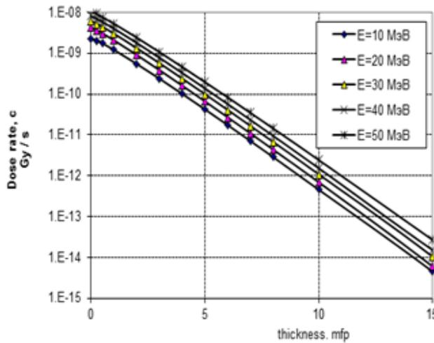
**Fig. 3.** Spatial distributions in Concrete of the power of the absorbed dose of photons in the air from flat unidirectional photon sources with different power
