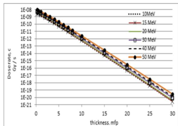
**Fig. 2.** Spatial distributions in Concrete of the power of the absorbed dose of photons in the air from point isotropic photon sources with different power energies 1 photon ./s (results multiplied by  $4\pi R^2$ )
