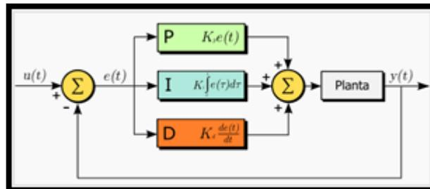
Figure 1. Block diagrams of a PID Control.
