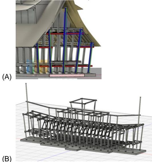
**Figure 3.** (A) Building poles (B) Construction of building poles totaling 72 pieces And connecting beams having the same model.
