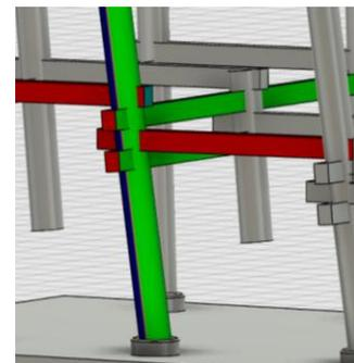
**Figure 5.** All supporting poles are joined without nails
