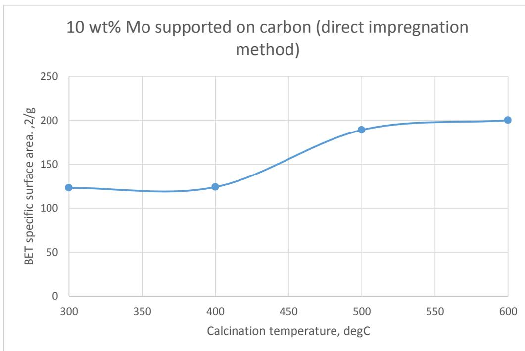
**Fig.2:** Effect of calcination on specific surface area of 10wt.% MoO<sub>x</sub> supported on carbon
