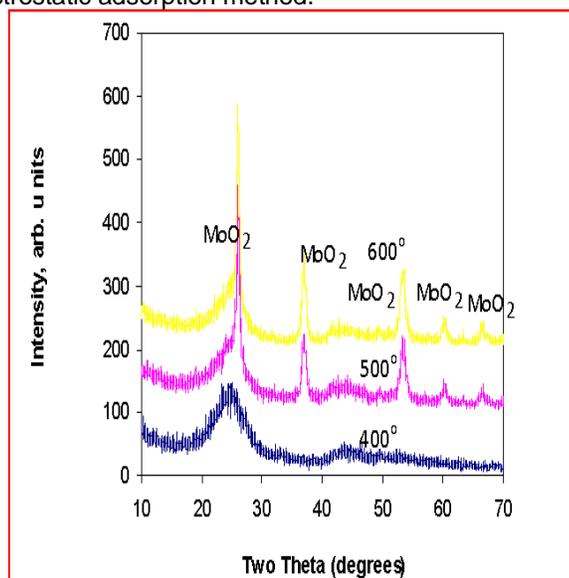
Fig.1: Powder XRD patterns with different calcination temperatures of  $\text{MoO}_x$  supported carbon
