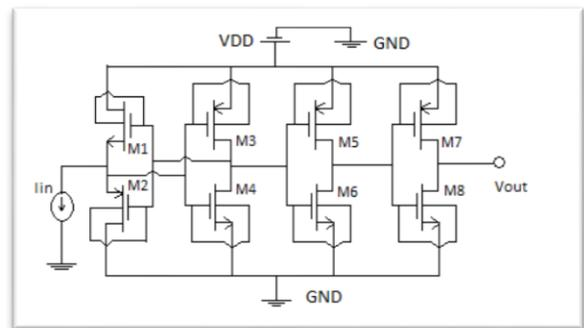
Figure 2 Proposed Current Comparator using DTMOS
