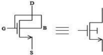
Figure 1 MOS transistor using DTMOS
