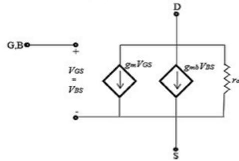
Figure 3 small signal model of DTMOS
