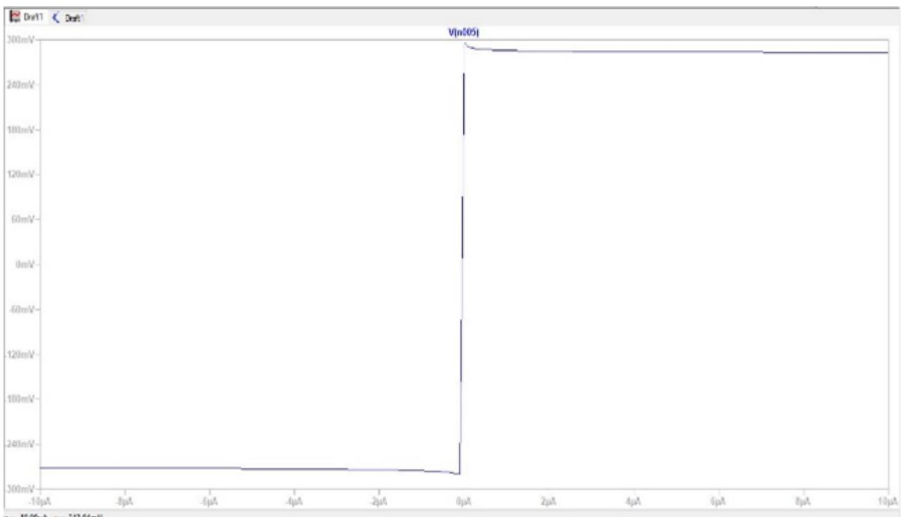
**Figure 6** DC response from proposed comparator
