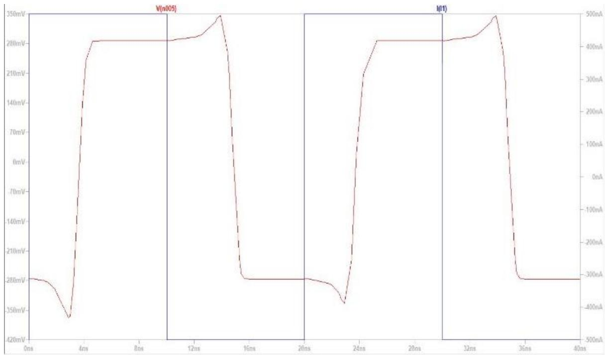
**Figure 5** Transient response of proposed comparator
