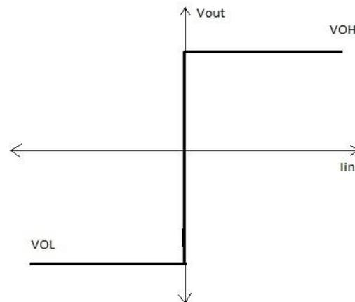
**Figure 1** Transfer Characteristics of an Ideal Current Comparator
