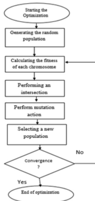
Fig 2. Genetic Algorithm Flowchart
