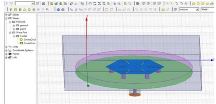
**Figure 6. Coaxial feed assignment to the designed 3D structure**
