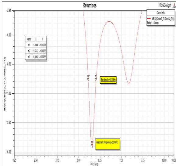
**Figure 11.** Return loss of designed hexagonal patch with Shorting pins
