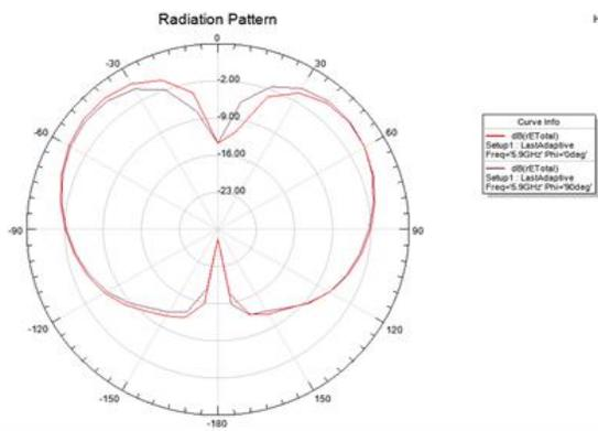
**Figure 12.** Radiation Pattern of designed hexagonal patch with Shorting pins
