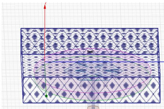
**Figure 5. Assigning radiation boundary to the designed 3D structure**
