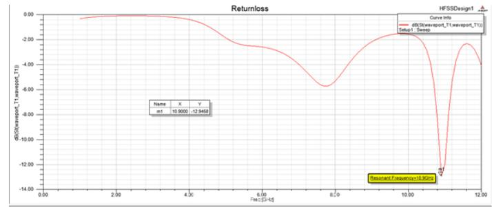
**Figure 9.** Return loss of designed hexagonal patch
