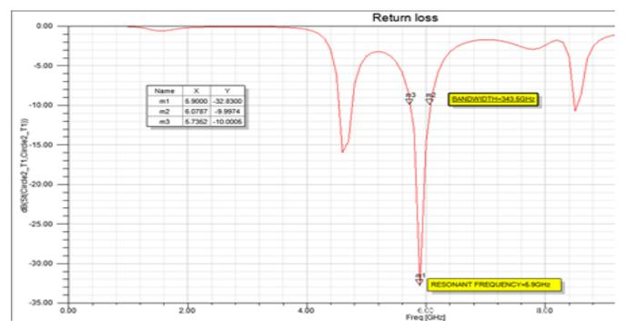
**Figure 15.** Return loss measurement with V shaped slots on overall design
