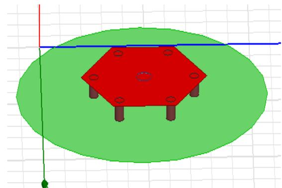
**Figure 10.** Shorting pins between patch and ground
