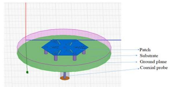
Figure 3. Creation of Geometry of the designed Antenna
