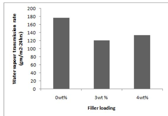
Figure 4. Water vapour transmission rates of PLA/AA with filler loading
