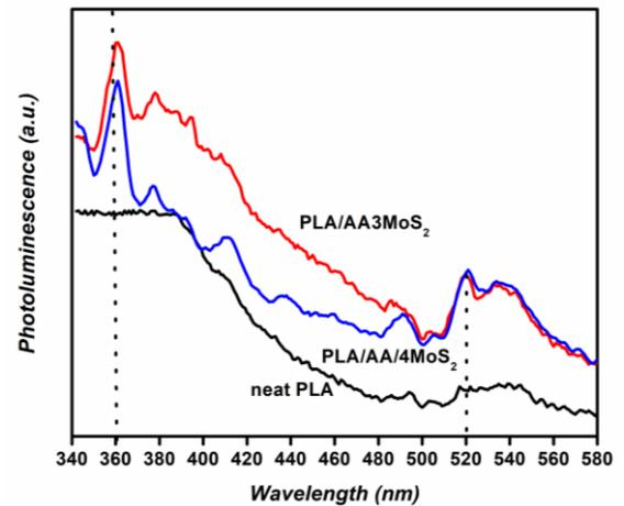
Figure 3. Photoluminescence spectrum of PLA and PLA/AA/MoS<sub>2</sub> composites
