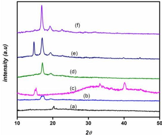
Figure 2. The Xrd spectrum of (a) VAA; (b) neat PLA; (c) LiMoS<sub>2</sub>; (d) PLA/AA1wt%MoS<sub>2</sub>; (e) PLA/AA/3wt%MoS<sub>2</sub>; (f) PLA/AA/4wt%MoS<sub>2</sub>
