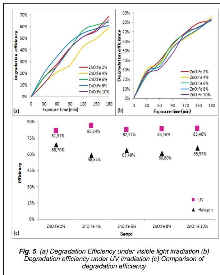
Fig. 5. (a) Degradation Efficiency under visible light irradiation (b) Degradation efficiency under UV irradiation (c) Comparison of degradation efficiency
