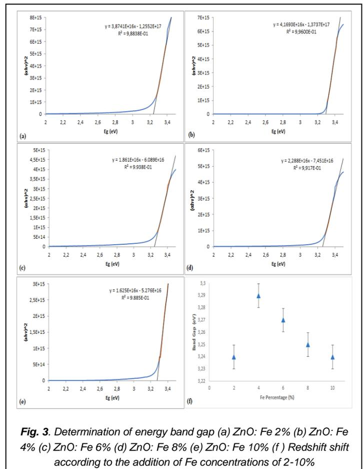
Fig. 3. Determination of energy band gap (a) ZnO: Fe 2% (b) ZnO: Fe 4% (c) ZnO: Fe 6% (d) ZnO: Fe 8% (e) ZnO: Fe 10% (f) Redshift shift according to the addition of Fe concentrations of 2-10%
