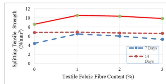
**Figure 7:** Textile Fabric Fibre Concrete splitting tensile strength at 7, 14 and 28 days.
