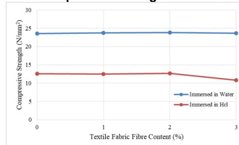
**Figure 10:** Textile Fabric Fibre Concrete compressive strength after immersion in acids for 27 days.
