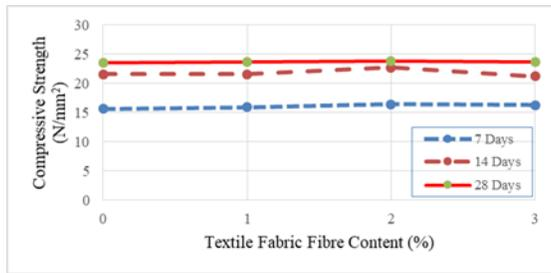
**Figure 3:** Textile Fabric Fibre Concrete compressive strength at 7, 14 and 28 days
