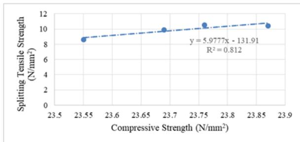
**Figure 8:** Relationship between compressive strength and splitting tensile strength at 28 days.
