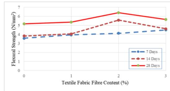
**Figure 5:** Textile Fabric Fibre Concrete flexural strength at 7, 14 and 28 days
