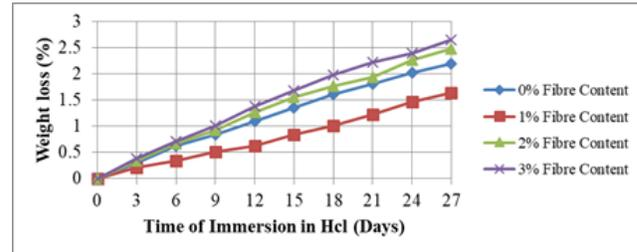
**Figure 9:** Rate of weight loss of Textile Fabric Fibre Concrete immersed in HCl over time.
