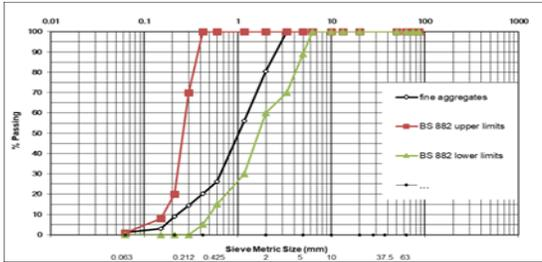
Figure 1: Particle size distribution of the fine aggregate
