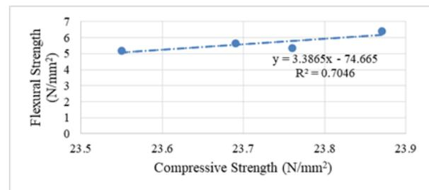
**Figure 6:** Relationship between compressive strength and flexural strength at 28 days.
