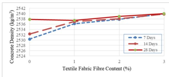
**Figure 4:** Textile Fabric Fibre Concrete cube density at 7, 14 and 28 days.
