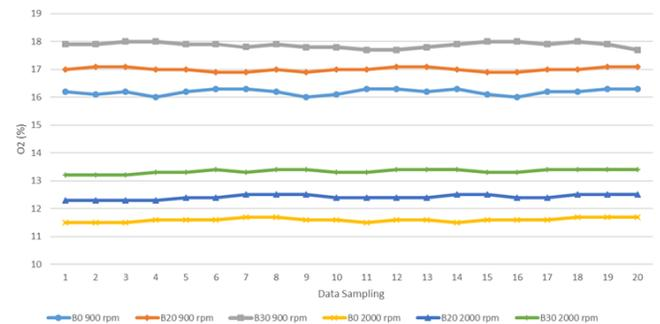
Figure 3. O<sub>2</sub> Gas comparison in Each Fuel Variant
