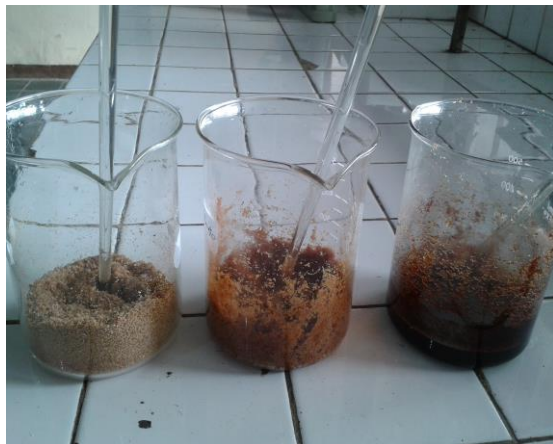
Fig. 1. From left to right: (i) glass of sawdust; (ii) liquefaction process; and (iii) liquefaction product
