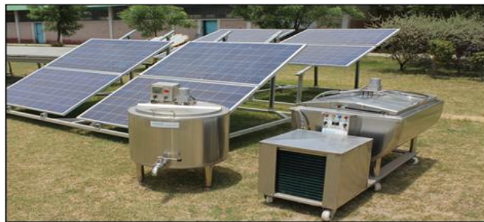
Fig. 1 Energy Efficient Solar Based Milk Chiller Unit
