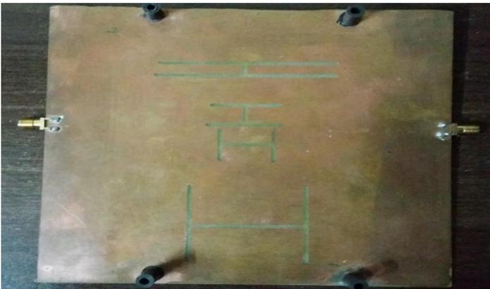
Figure 10-3: Coupling Slots on Ground Plane of Antenna
