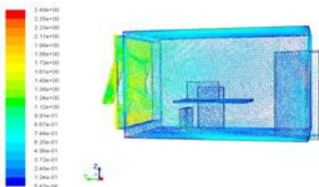
Fig. 5. Distribution of velocity in the office at 8:00 am
