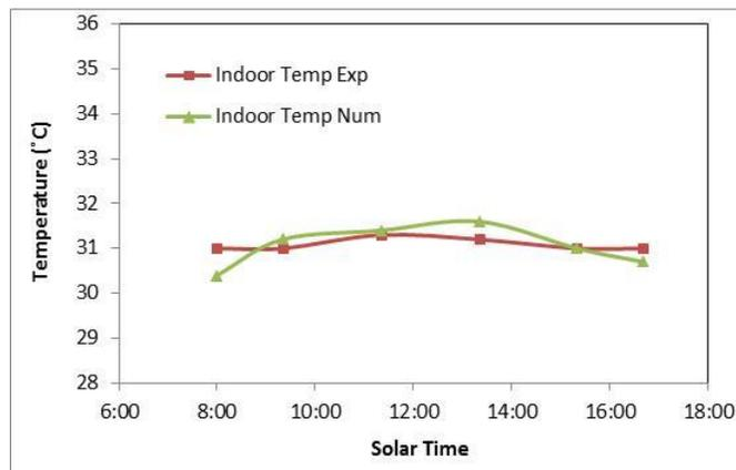
Fig. 7. Averaged Temperature comparison between measurement data and CFD
