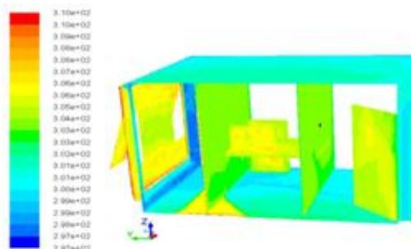
Fig.6. Distribution air temperature in the office at 8:00 am
