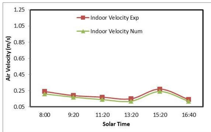
**Fig. 8.** Air velocity comparison between measurement data and CFD
