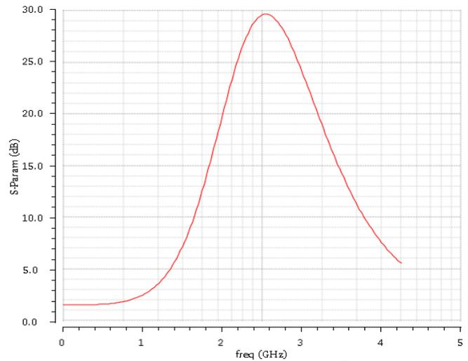
**Fig. 7** Simulated voltage gain  $S_{21}=30\text{dB}$  @ 2.4GHz center frequency
