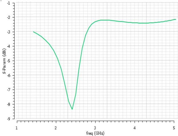
**Fig. 10** Simulated input return loss  $S_{11}$  = -8.4dB @ 2.4GHz center frequency
