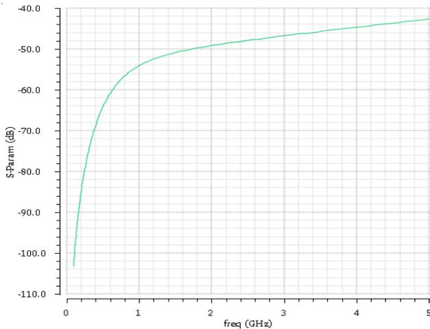
**Fig. 9** Simulated reverse isolation ( $S_{12}$ ) = -48dB @2.4GHz center Frequency
