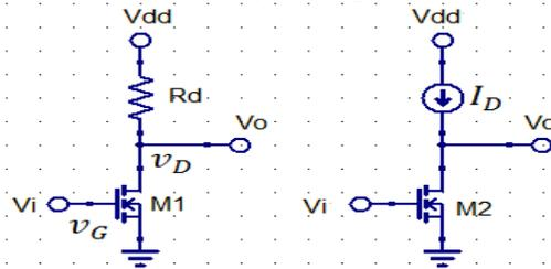
Fig. 1. Single transistor amplifier
