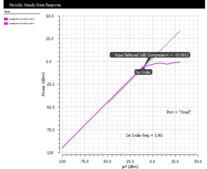
**Fig. 12** The simulated 1dB Compression point ( $P_{1dB}$ ) = -10.6dBm
