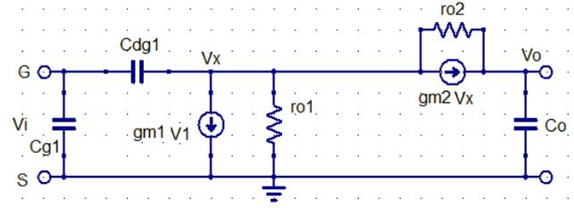
Fig. 3. The small- signal model analysis for cascode.
