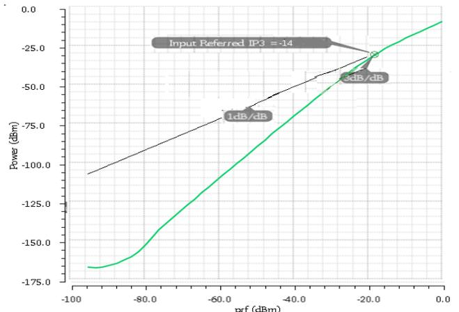
**Fig. 13** The simulated  $IIP_3$  = -14dBm
