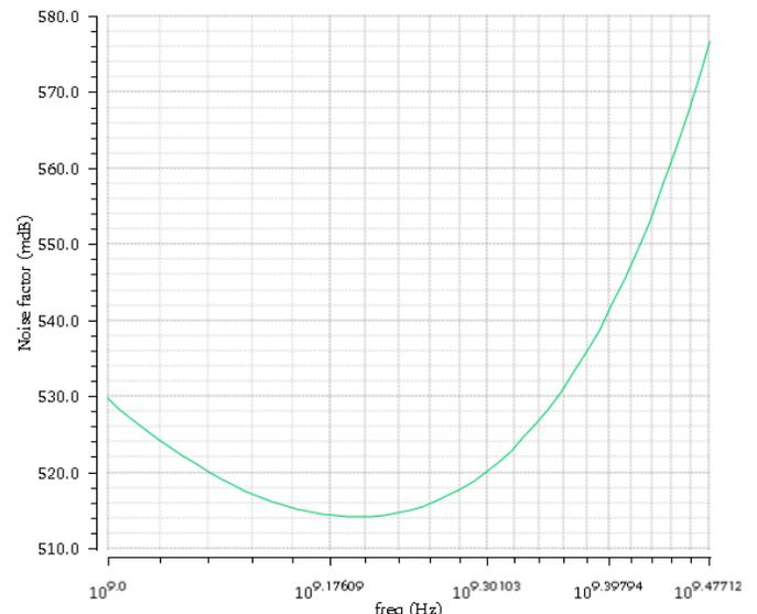
**Fig. 8** Simulated noise figure (NF) = 0.54dB @ 2.4GHz center frequency
