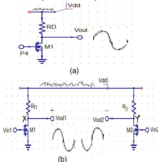
Fig. 5. Noisy signals for (a) single-ended (b) differential paths
