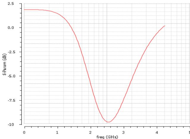
**Fig. 11** Simulated output return loss  $S_{22}$  = -10dB @ 2.4GHz center frequency
