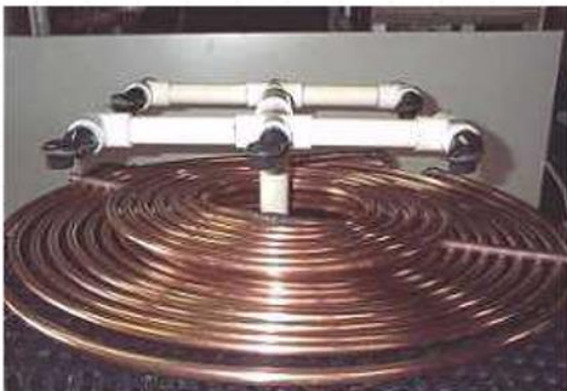
Figure (3) Water Cooled Condenser layout
