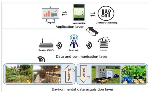
**Figure 6: Architecture: A Control System.**
