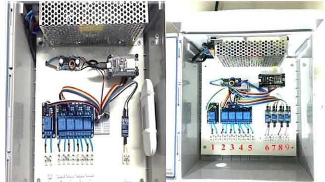
**Figure 7: Set-up: A control box design.**
