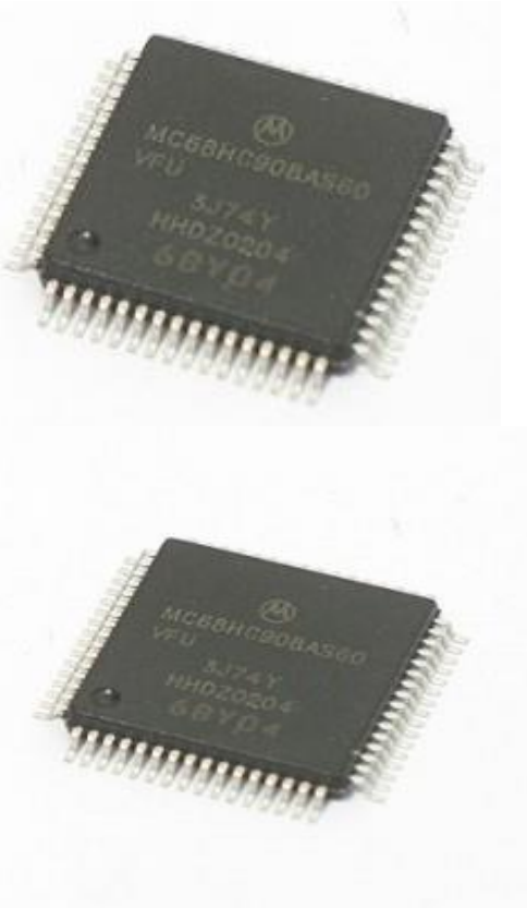
Fig5. Micro Controller Unit
