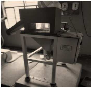
Fig 4: Lab set up of jigging of M/s. Insmart systems, Hyderabad
