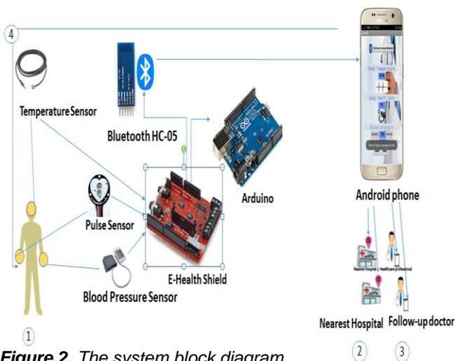
Figure 2. The system block diagram.
