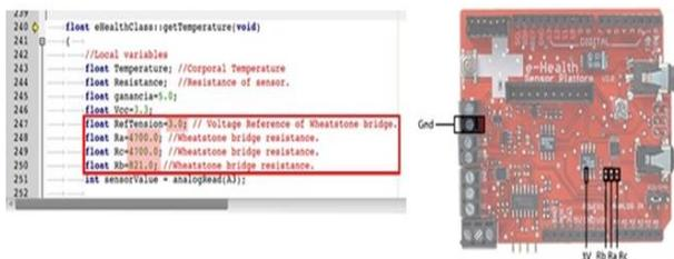
Figure 8. The calibration of the temperature sensors.
