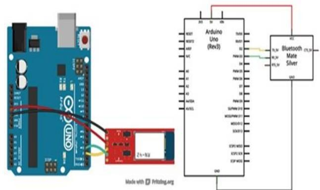
Figure 6. The connection between Bluetooth and the Microcontroller
