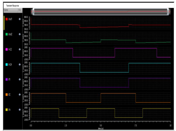
**Fig. 15.** Simulated results of top module for signal decompression
