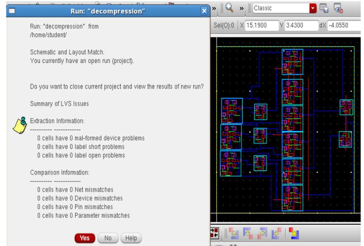
**Fig. 14.** Decompression top module layout design with LVS results
