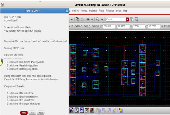
**Fig. 11.** Top module layout design with LVS results
