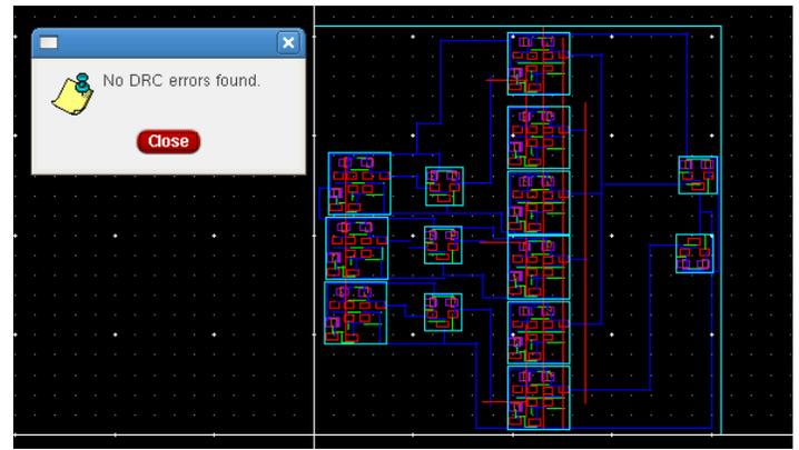
**Fig. 13.** Decompression top module layout design with DRC results
