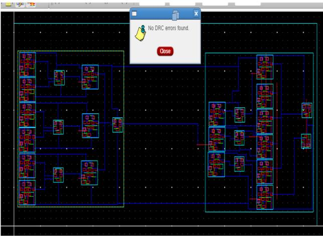
**Fig. 10.** Compression top module layout design with DRC results
