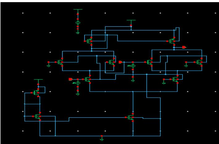
**Fig.8 (a).** Schematic circuit of Gilbert cell multiplier factor and its simulated results
