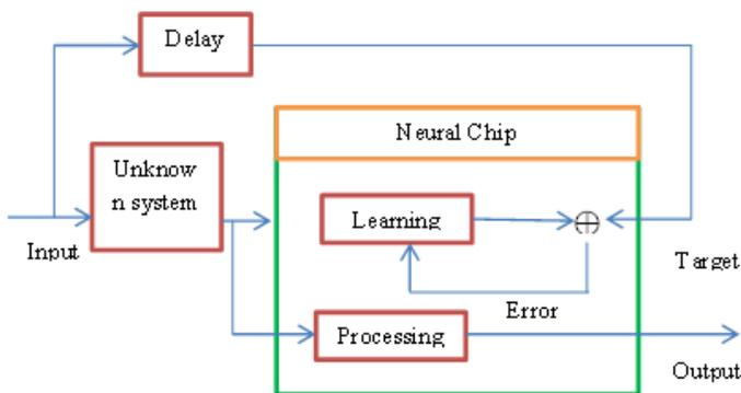
**Fig.3.** Design of Inverse Modeling to monitor the target output
