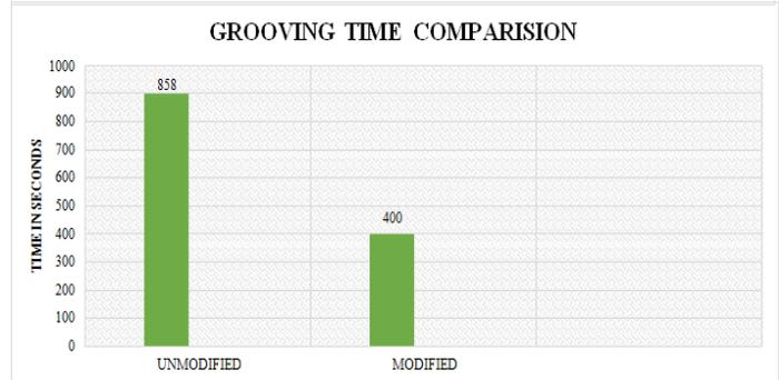
required to change the fixture for another model pad thus increasing the productivity in the line. With the inclusion of the positive chamfer in the preform and curing moulds, the entire process of chamfering for the disk pads is eliminated in the finishing line. The pads with chamfer length greater than 15mm avail this feature in their preform and curing moulds. The useful man time of about 121 seconds could be saved.
