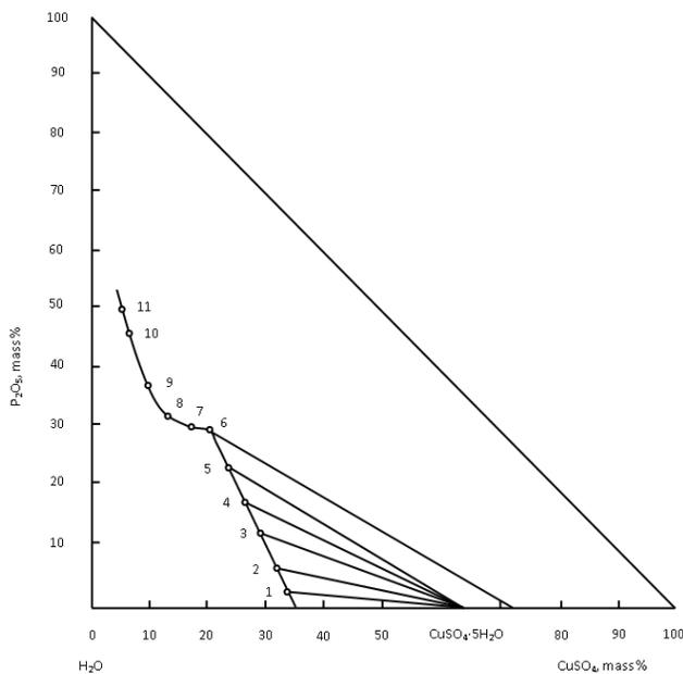
**Fig. 4.** The solubility isotherm of the  $\text{CuSO}_4\text{-H}_3\text{PO}_4\text{-H}_2\text{O}$  system at  $80^\circ\text{C}$
