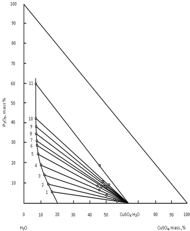
**Fig. 1.** The solubility isotherm of the CuSO<sub>4</sub>-H<sub>3</sub>PO<sub>4</sub>-H<sub>2</sub>O system at 30 ° C
