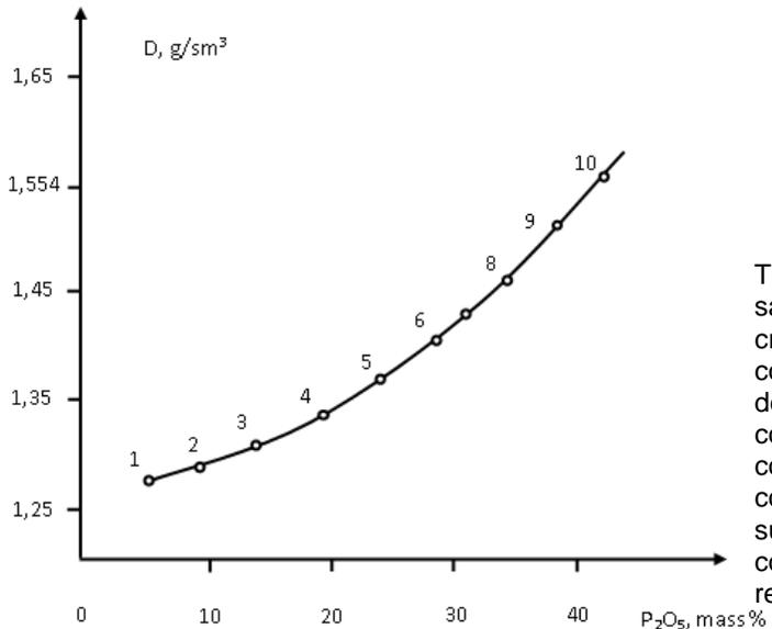
**Fig. 3.** Change in the density of saturated solutions in the  $\text{CuSO}_4\text{-H}_3\text{PO}_4\text{-H}_2\text{O}$  system at  $30^\circ\text{C}$
