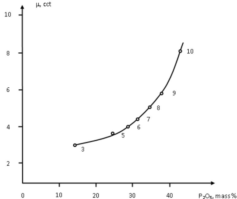
**Fig. 2.** The change in the viscosity of saturated solutions in CuSO<sub>4</sub>-H<sub>3</sub>PO<sub>4</sub>-H<sub>2</sub>O at 30 ° C
