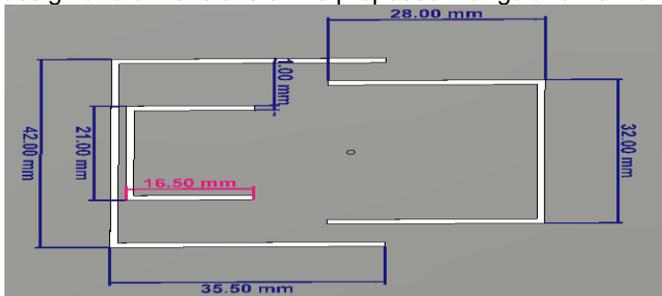
Fig. 2. Dimensions of the proposed antenna
