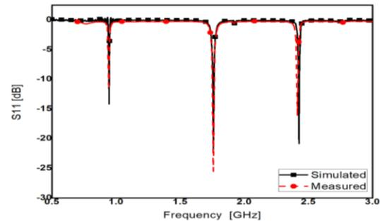
Fig. 7. Measurement and simulation of the reflection coefficient
