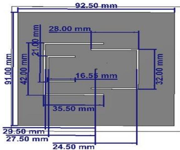
Fig. 1. triple-unit antenna.
