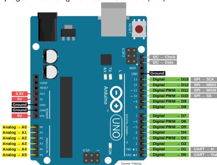
**Fig. 2. Arduino Uno Pinout**
