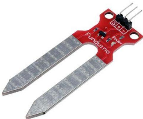
**Fig. 3. Soil Moisture Sensor**
