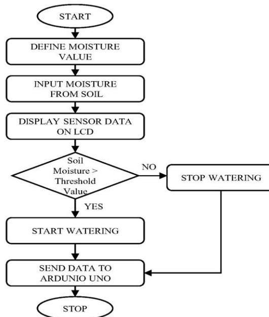
Fig. 7. Water Controlling Flowchart
