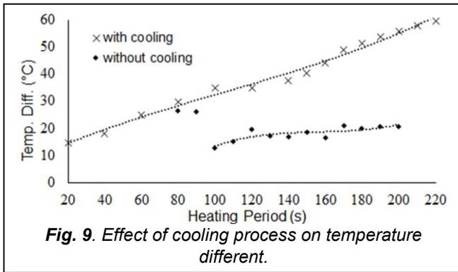
**Fig. 9.** Effect of cooling process on temperature different.
