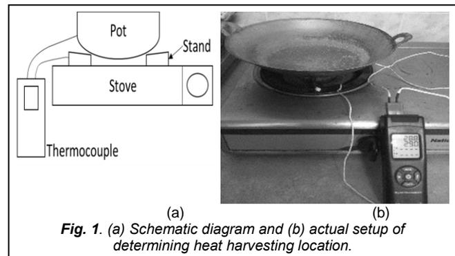
Fig. 1. (a) Schematic diagram and (b) actual setup of determining heat harvesting location.
