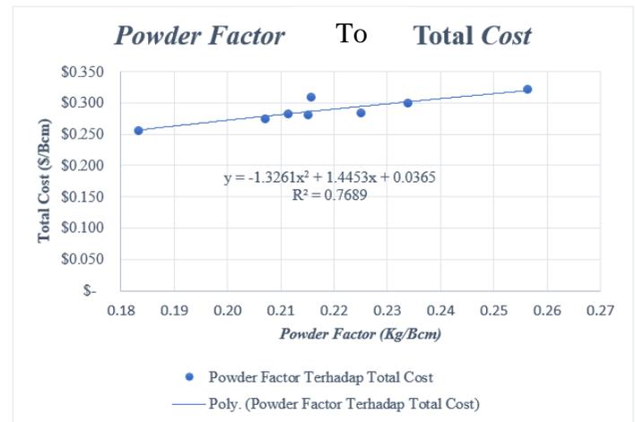
**Figure 5.** Graph of equations between PF and total blasting costs.
