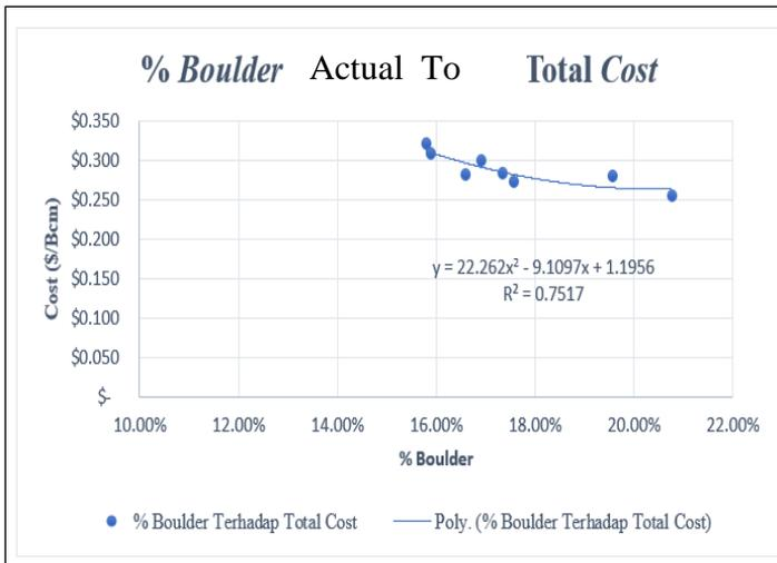
**Figure 4.** Graph of the equation between the percent of actual boulder and the total cost of blasting.
