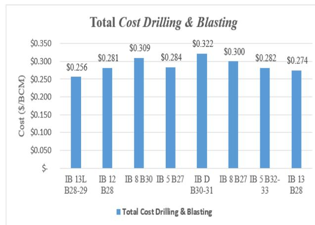
**Figure 3.** Graph of total drilling and blasting costs for each blasting activity.
