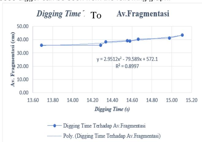
**Figure 2.** Graph of the relationship between digging time of the digging tool for each blasting activity material with the average fragmentation.
