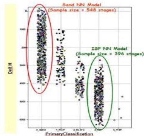
Figure 8. Proppant Type as Function of Depth Below Top of Productive Interval (DeltH)
