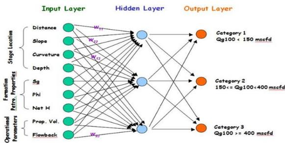
Figure 7. FeedForward Neural Network with Geologic, Petrophysical, and Operational Parameter Input Variables and Categorical Qg100 Output Variables
