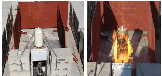
Fig. 5. A real fire test for a gas cylinder without a firewall
