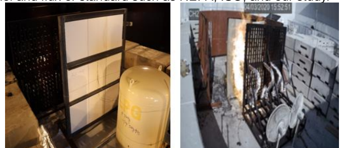
Fig. 6. A real fire test for a firewall between an LPG tank and a burner.
