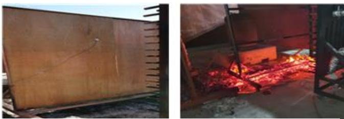
Fig. 7. Photographs of a firewall(LWD) before and after experiments.
