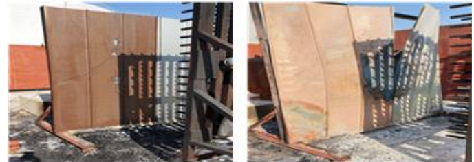
Fig. 9. Photographs of a firewall(EPS) before and after experiments.
