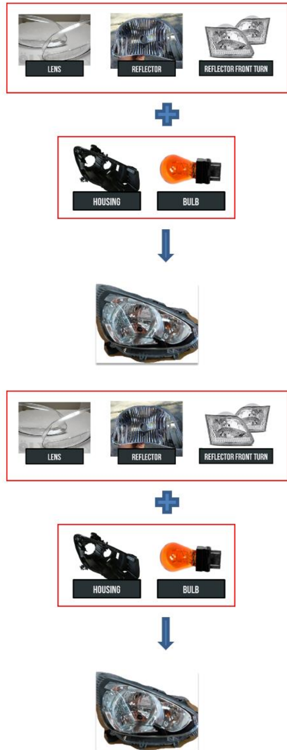
Fig. 2. Outline flow process chart of a headlamp production
