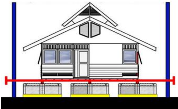
Fig 6. The illustration of the application of the TAM foundation in house construction
