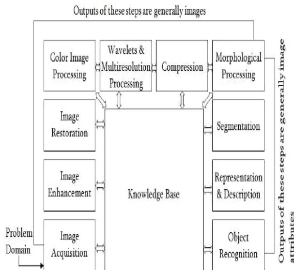
**Figure 1.** Architecture of image processing and function involved.
