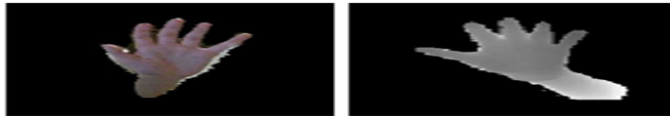
Fig. 6. Illustration of data obtained using Kinect. (a) RGBcolor image of the hand region (b) Depth image of the hand region
