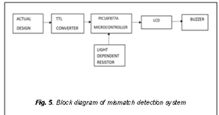
Fig. 5. Block diagram of mismatch detection system
