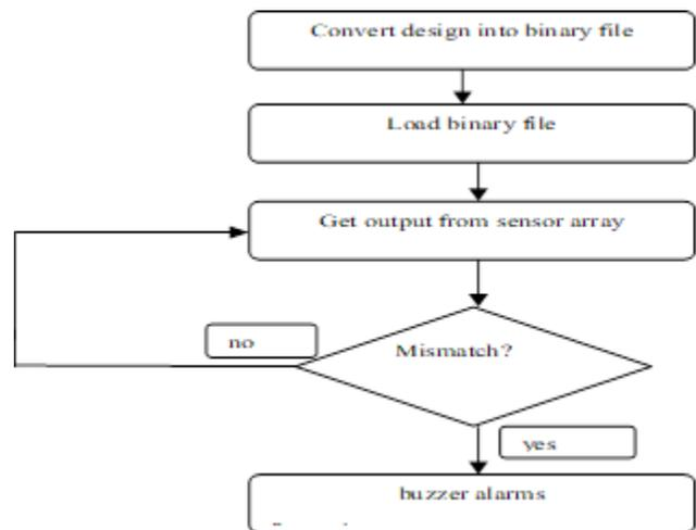
Fig. 6. Flowchart of mismatch detection system
