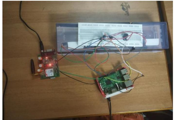
**Figure 3.3 GSM interfaced with Raspberry Pi**
