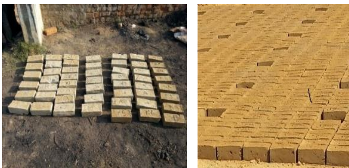
(a) Drying of Bricks (b) Bricks before heating Fig 3 Photo view of Drying of Bricks Used
