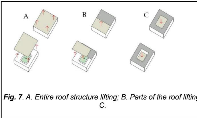
**Fig. 7.** A. Entire roof structure lifting; B. Parts of the roof lifting; C.
