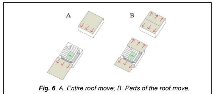
Retractable roof with lifting system could be lifted and lowered to desired height.
