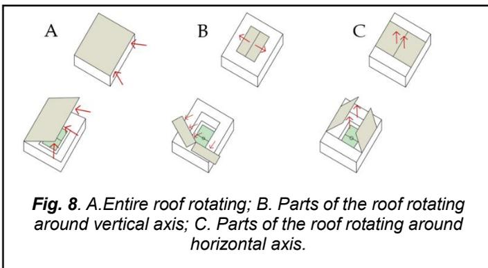
**Fig. 8.** A. Entire roof rotating; B. Parts of the roof rotating around vertical axis; C. Parts of the roof rotating around horizontal axis.
