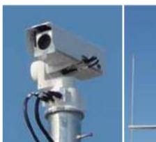
Fig 3: 360 degree rotating camera
