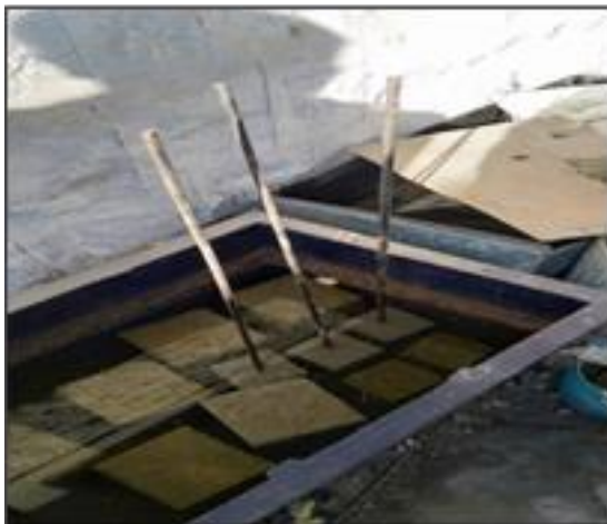
Fig.8 Curing of cubes
