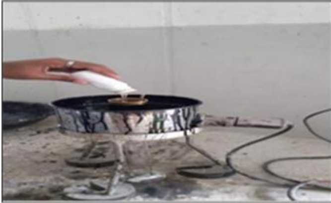
Fig. 5 Viscosity test on Polyvinyl Alcohol gel
