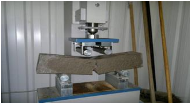
Fig 6 Flexure Strength Of Beam
