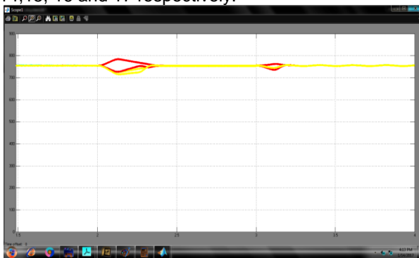
Fig.12 DC capacitor voltages of AC/DC converter by the proposed method
