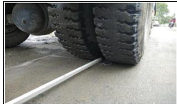
Fig .4 Setting up BBD test apparatus and taking deflection measurements.
