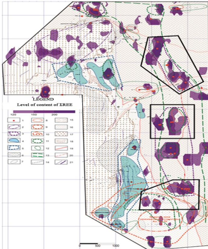
Fig 9. Schematic forecast-geochemical map of the Eastern Altyntau section (10,606 samples from primary geochemical halos). (Compiled by S.M. Koloskova).
