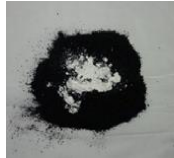
Figure 3.14. Mixing the coconut charcoal powder with Sodium Carbonate into 3 parts then stir with a plastic bag for 15 minutes
