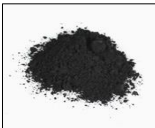
Figure 3.12 15gr of coconut shell charcoal powder
