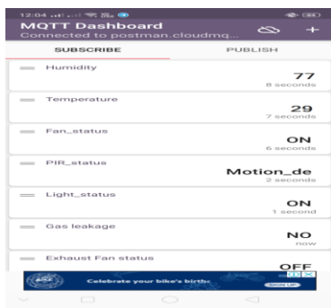
Fig. 15. Cloud MQTT Dashboard showing Motion Detected, ON status of the Light, Temperature and Humidity information
