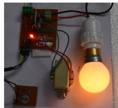
Fig. 24. Case 2: Medium Room Brightness then Bulb glows with Normal Brightness
