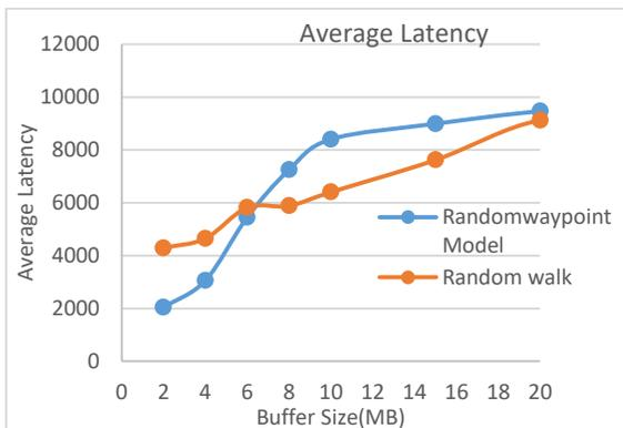
Figure 6 (b) Average Latency of epidemic routing protocol for varying Buffer size with the message size 1MB
